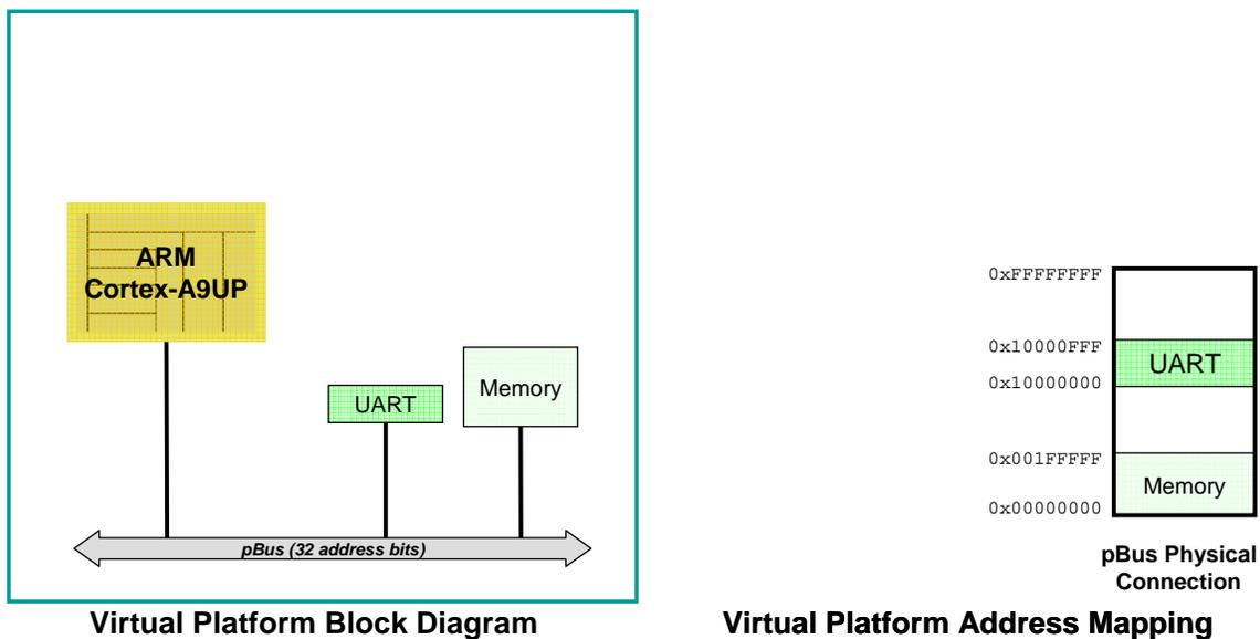
Figure 1: Platform 'ignoreTrustZone' Block Diagram and Memory Mapping
