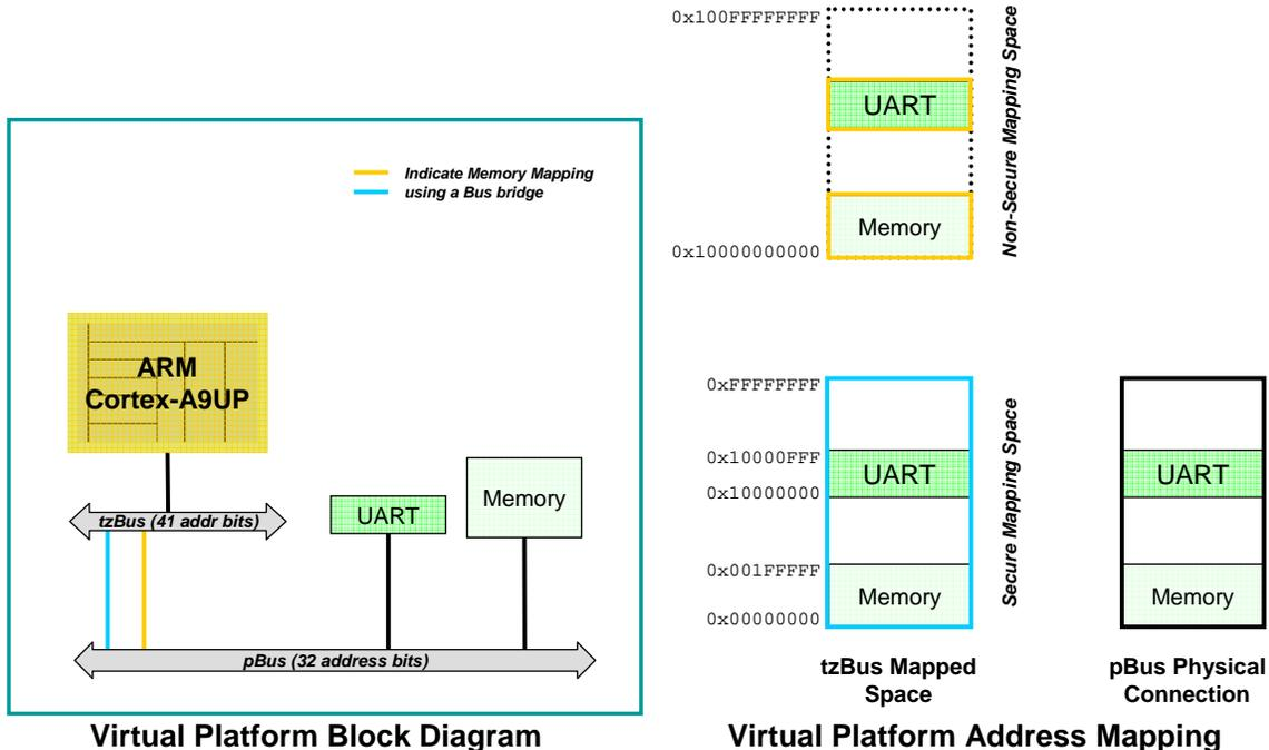
Figure 3: Platform 'alwaysNonSecure' Block Diagram and Memory Mapping
