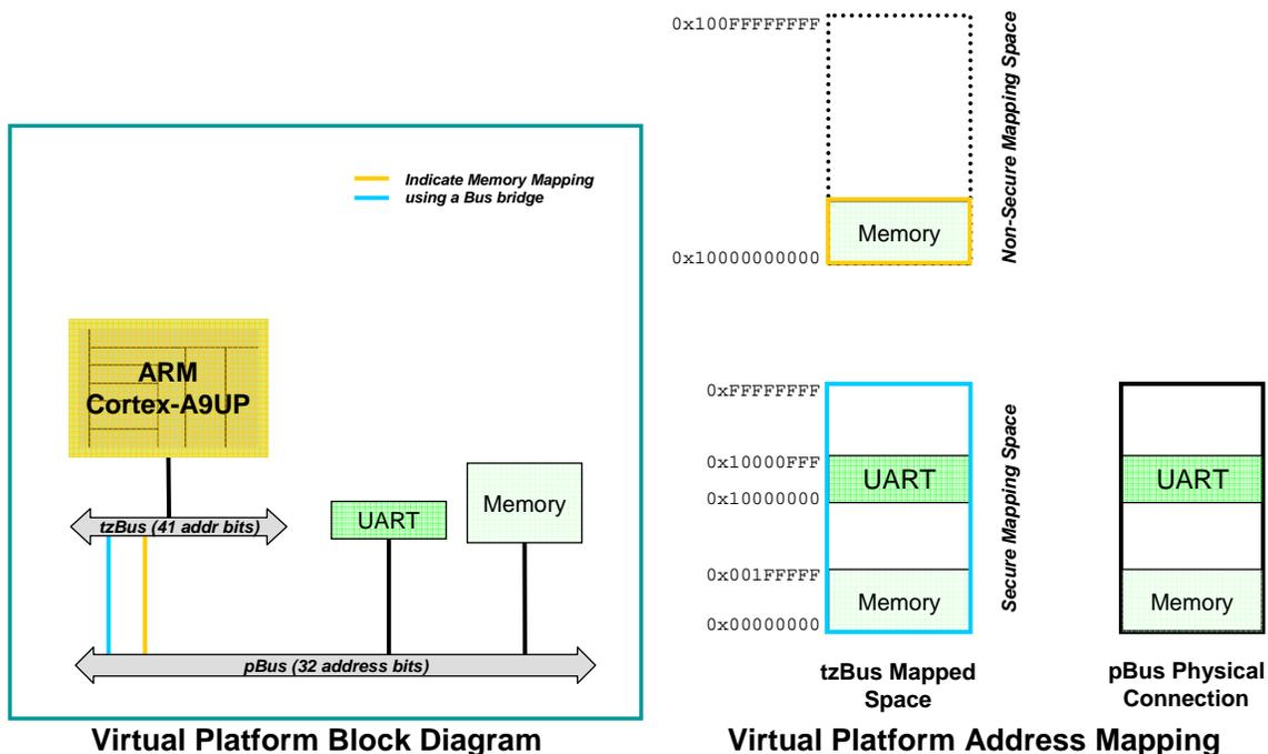
Figure 2: Platform 'alwaysSecure' Block Diagram and Memory Mapping
