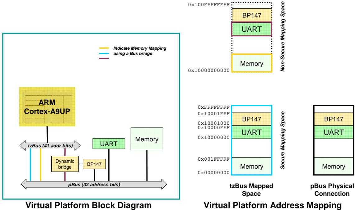
Figure 4: Platform 'programControl' Block Diagram and Memory Mapping
