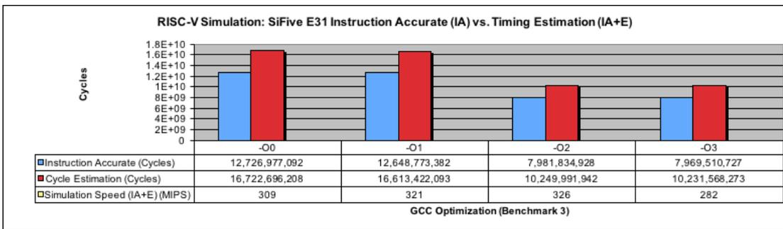
Fig. 6. IA+E cycle estimation results for the SiFive E31 processor.
