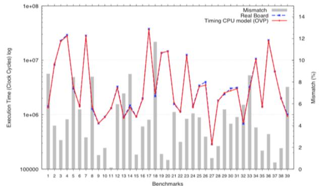
Fig. 3. Timing estimation results for IA+E simulation show average errors of better than +/- 5% over 39 different benchmarks for Arm Cortex-M4.
