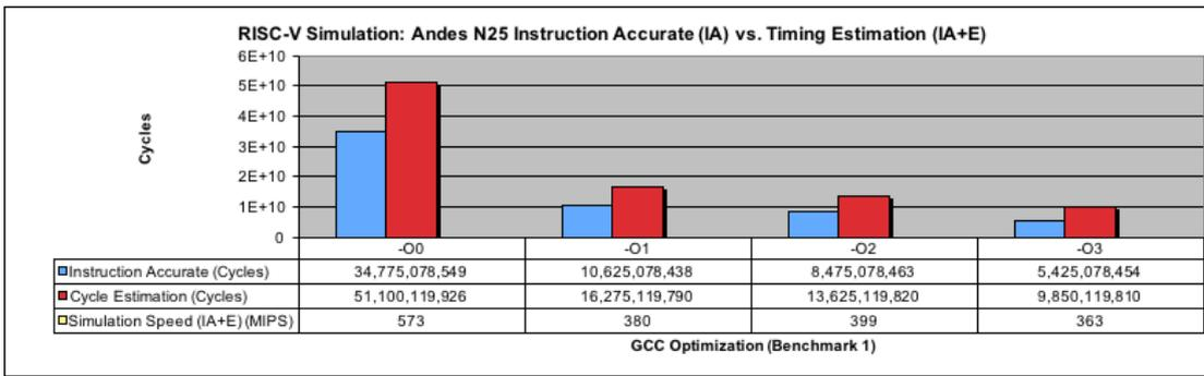
Fig. 4. IA+E cycle estimation results for the Andes N25 processor.
