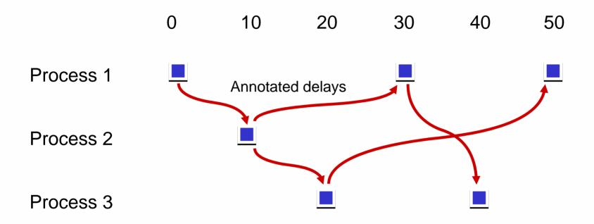
Each process is synchronized with SystemC scheduler Delays can be accurate or approximate
