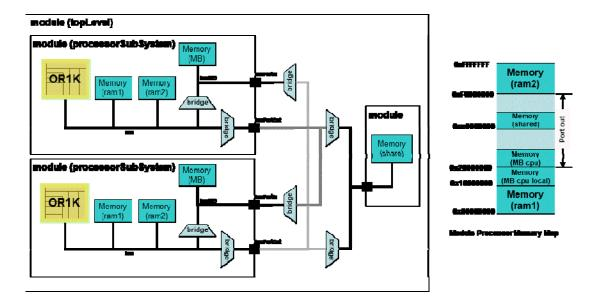
The top level instances the other modules of the design and creates the interconnecting bus. This is defined in *topLevel/module.op.tcl*:
