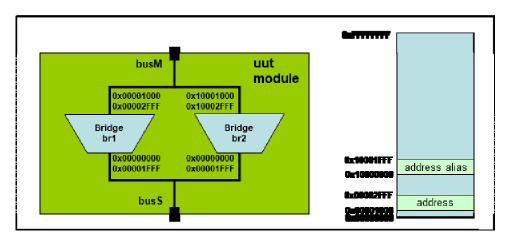
An alternate method, and recommended as this overcomes a failure in SystemC, is to create a second bus on which the components and memory are located separately to the bus masters which see the aliased memory. This requires the use of two bus bridges, one to make the original mapping and the second to make the aliased mapping.
