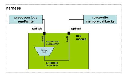
In this example a processor read/write in the address range 0x00001000 to 0x00002fff will be mapped to a memory access in the range 0x10000000 to 0x10001fff.
